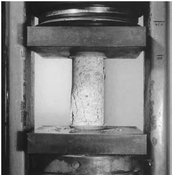
Figure 25.12 – Testing a Cylinder for Compressive Strength
