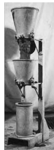
Figure 25.6 – The Compacting Factor Test Apparatus
